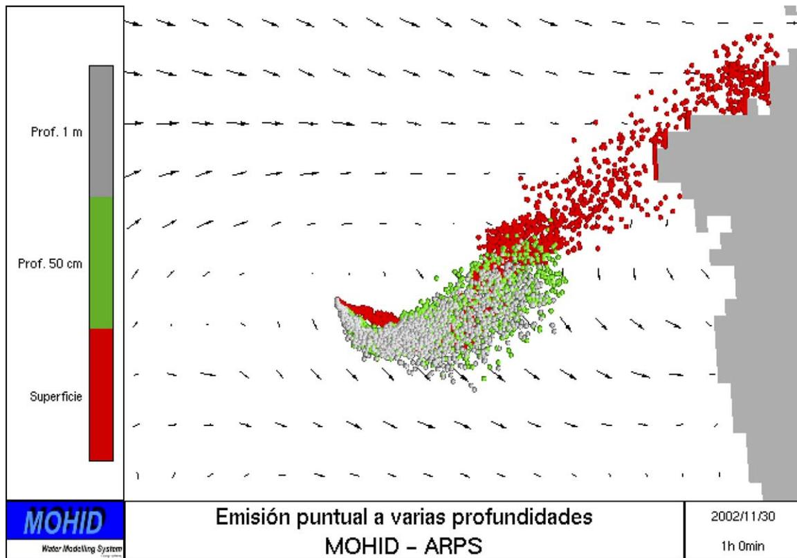
Fig. 6. METEOMOHID simulation of the main spill track taking into account the slope current. Oil displacement was computed adding to the barotropic currents the baroclinic ones obtained with November climatologic temperature, salinity fields. Red lagrangian tracers indicate surface tracers, green ones represent 0.5 m depth tracers and the grey ones are tracers at 1 m depth.
