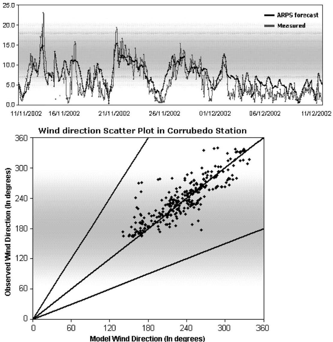
Fig. 2. Comparison of ARPS output wind data for the nearest grid point against data from automatic meteorological station at Corrubedo.
