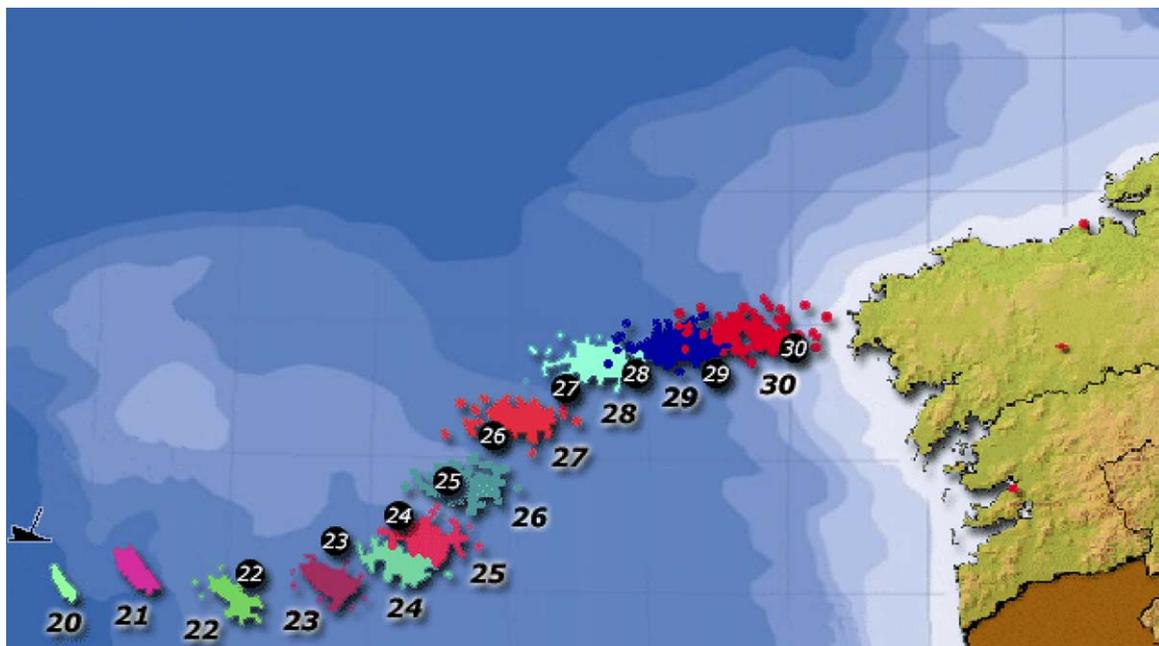
Fig. 5. METEOMOHID simulation of the main spill track. Comparison of the forecasted position (coloured spots) with overflight observed position (black circles).
