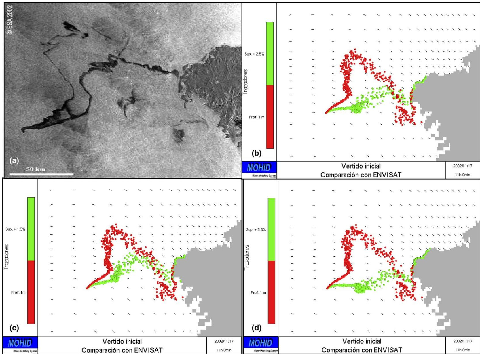
Fig. 4. Tracers are released at different depths: surface tracers (red), 1 m depth tracers (green). Surface tracers are directly pulled by wind with a velocity proportional to the wind velocity in a percentage of (b) 1.5%, (c) 2.5%, (d) 3.3%. Results are compared with ENVISAT satellite image (a) taken on November 17th. (For interpretation of the references in colour in figure legends, the reader is referred to the Web version of this article.)
